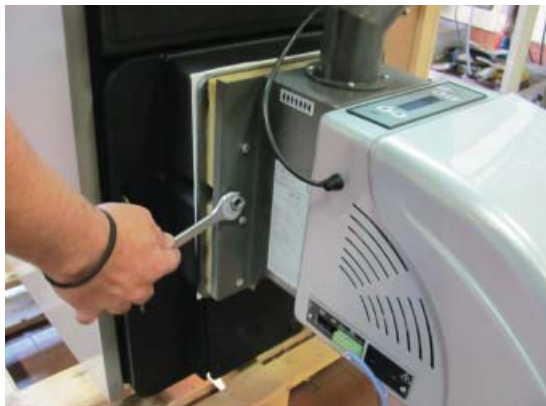
Fig. 25 Burner assembly
