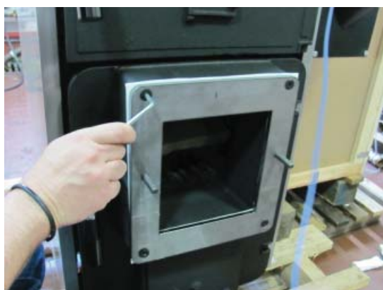
Fig. 23 Plate fixed to the combustion chamber door
