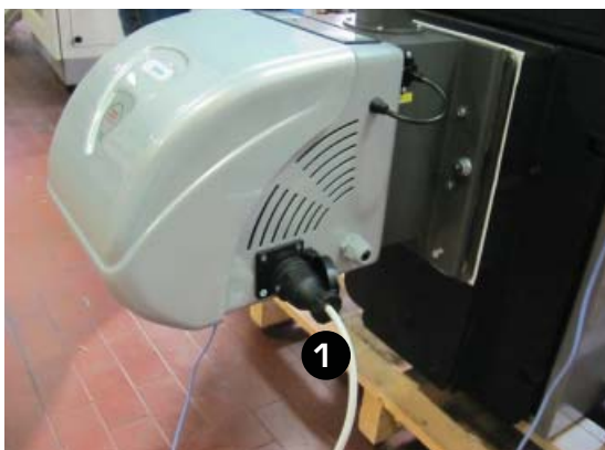
Fig. 33 Screw feeder motor cable
