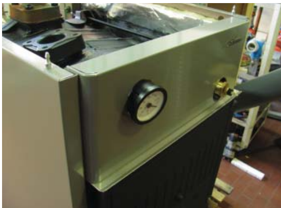
Fig. 29 Remove the thermometer
